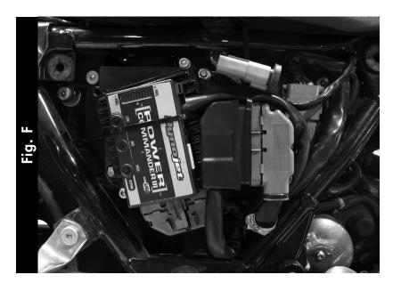
The unit can also be installed as in Fig. F. Use a zip tied to hold the connectors in place.
