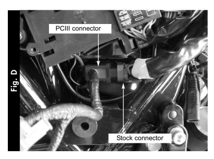
5 Remove the backing from the velcro and mount connectors to the bottom side of the battery tray (Fig. D).
