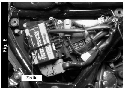
6 Plug the grey connector from the PCIII into the ECM.
