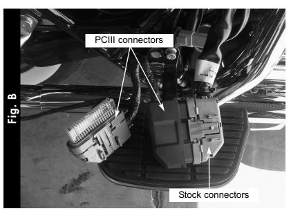
Plug the black connector from the PCIII into the stock wiring harness (Fig. B).
