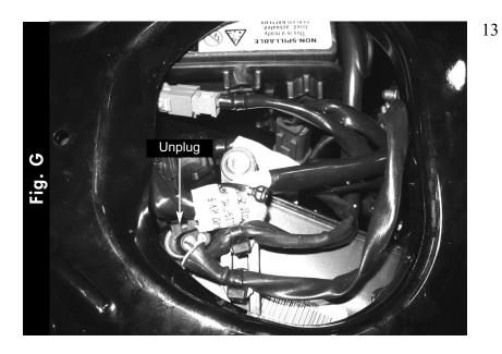
Unplug the rear O2 sensor from the stock wiring harness (Fig. G). This connector is located in the frame opening below the seat.
