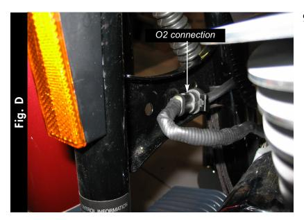
Disconnect the front O2 sensor from the main wiring harness (Fig. D).
