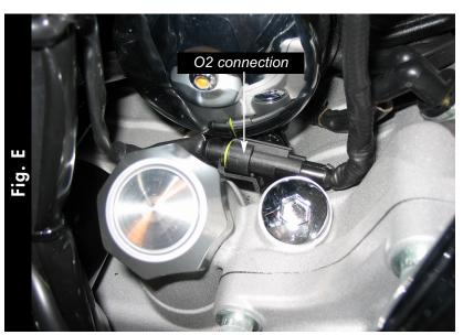
Disconnect the rear O2 sensor from the main wiring harness (Fig. E).
