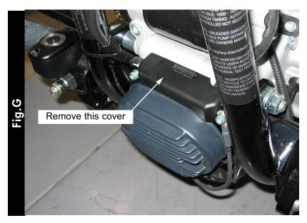
Remove the cosmetic cover on the front of the engine (Fig.G)
