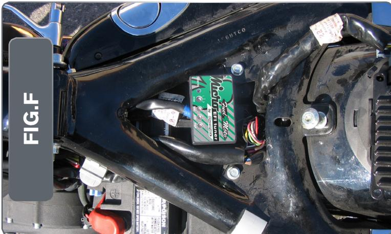
11 Install the Micro EFI Tuner module under the seat (Fig. F).
