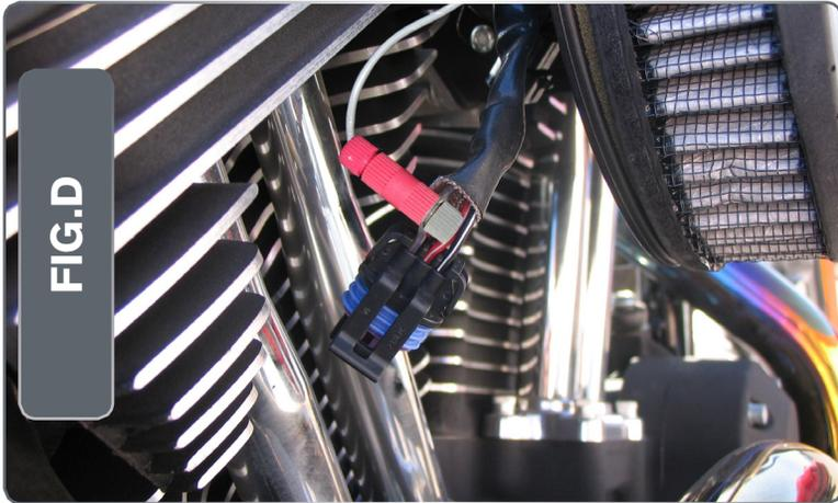
5 Unplug the stock Throttle Position Sensor connector from the bike's TPS.
