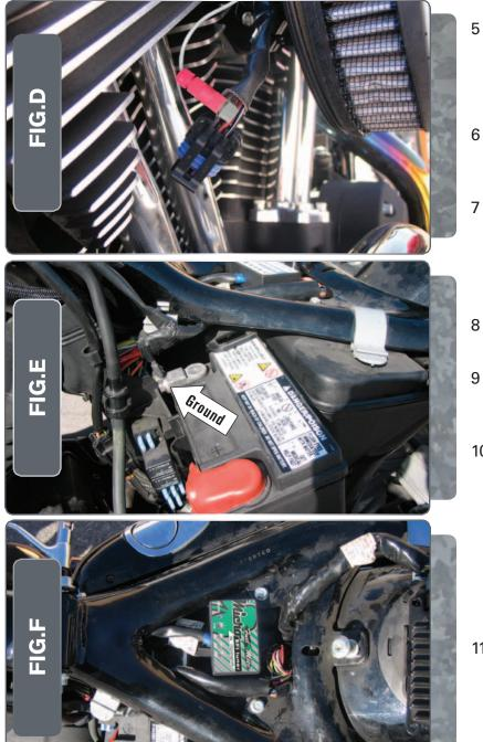
Unplug the stockThrottle Position Sensor connector from the bike'sTPS.
