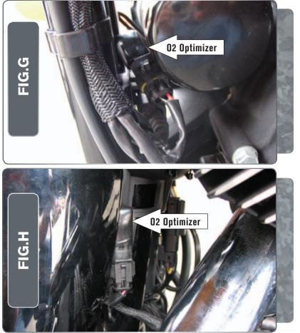
12 Locate and unplug the front O2 sensor connector.
