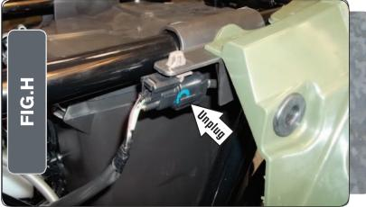
Just left of the airbox, locate and unplug the stock connectors for the ATV's O2 sensor (Fig. H).
