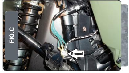
Inside of the right-rear fender well, secure the MicroTuner ring lug to the common ground bolt on the frame (Fig. C).
