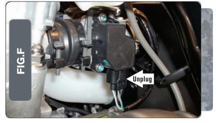
7 At the left side of the throttle body, unplug the stock wiring harness from the ATV's Throttle Position Sensor (Fig. F).
