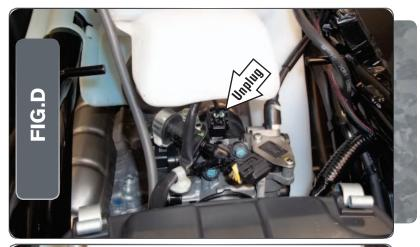
At the top of the throttle body, unplug the stock wiring harness from the ATV's Fuel Injector (Fig. D).
