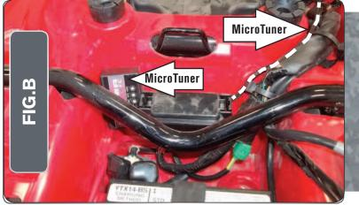
2 Using the supplied Velcro, secure the MicroTuner module towards the front of the battery compartment.
