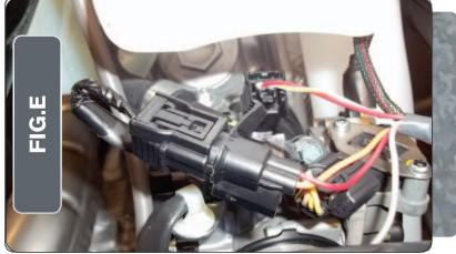
Plug the MicroTuner wiring harness in-line of the Fuel Injector and the stock wiring harness (Fig. E).
