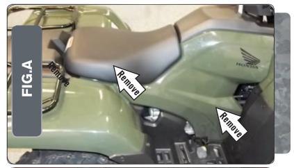
Remove the seat, the battery cover rear of the seat, and the body panels surrounding the ATV's fuel tank (Fig. A).
