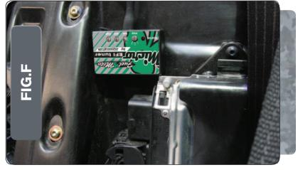
Using the supplied velcro, secure the MicroTuner to the panel behind the drivers seat above the ECU as shown in Figure F.
