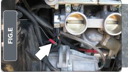
8 Using the supplied posi-tap, attach the grey wire from the MicroTuner to the green wire of the stockThrottle Position Sensor (TPS) harness as shown in Figure E.
