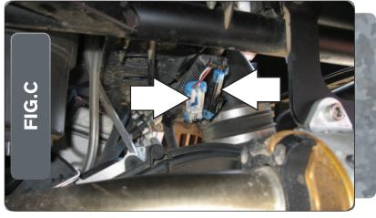
6 Unplug the sub connectors from each injector.
