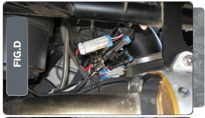
Attach the connectors from the MicroTuner to the stock wiring harness as shown in Figure D.
