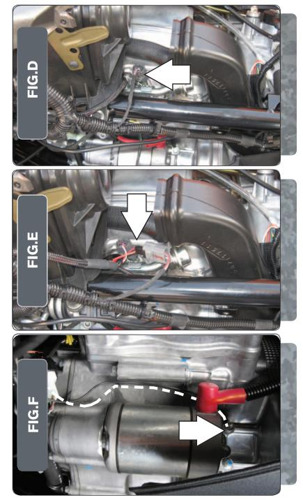
Unplug the stock wiring harness from the fuel injector as shown in Figure D.
