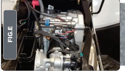
7 Attach the connectors from the MicroTuner harness to the stock wiring harness and the injector as shown in Figure E.
