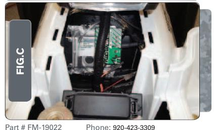
Using the supplied velcro, secure the MicroTuner on top of the stock ECU as shown in Figure C.
