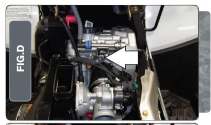
Unplug the stock wiring harness from the injector as shown in Figure D.
