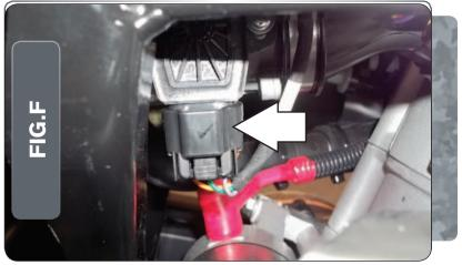
Unplug the stock wiring harness from the Throttle Position Sensor 8 (TPS) as shown in Figure F.
