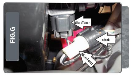
Attach the connectors from the MicroTuner harness to the stock wiring harness and TPS as shown in Figure G.
