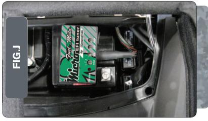
13 Using the supplied velcro, secure the MicroTuner to the battery as shown in Figure I.
