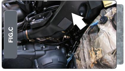
Remove the intake tube for the CVT clutch on the right hand side of the quad as shown in Figure C.
