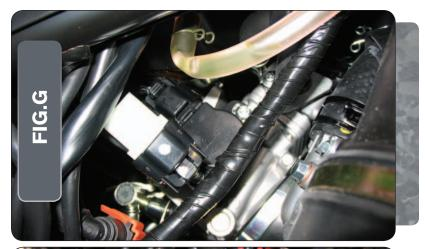
11 Attach the wiring harness from the MicroTuner to the stock wiring harness and the TPS as shown in Figure G.
