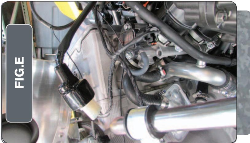
6 Plug the MicroTuner wiring harness in-line of the TPS and the stock wiring harness (Fig. E).
