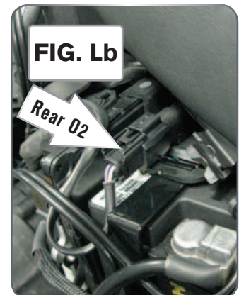
On Sportsters the front O2 connection is always at the front of the engine on the left side near the oil filter (Fig. La). The rear O2 connection is above the battery on 2014-2015 models (Fig. Lb) or just rear of the engine on 2007-2013 models (not pictured).
