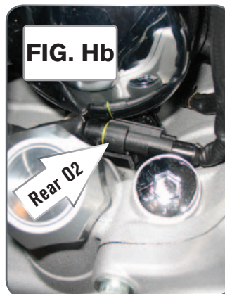
On 2007-2009 Touring models and 2007-2011 Softails the stock O2 connectors for the front cylinder are found at the front of the engine near the voltage regulator (Fig. Ha), and the rear cylinder O2 sensors connectors are found at the rear of the engine near the oil tank (Fig Hb).
