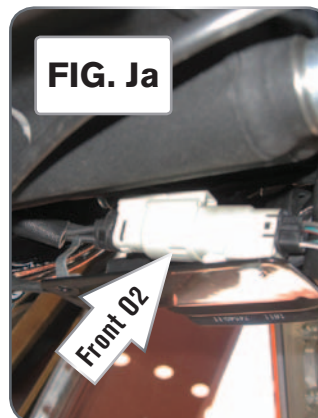
On 2012-2015 Softails the stock O2 connectors for the front cylinder are found at the front of the engine near the voltage regulator (Fig. Ja), and the rear cylinder O2 sensor connectors are found under the seat near the battery (Fig Jb).
