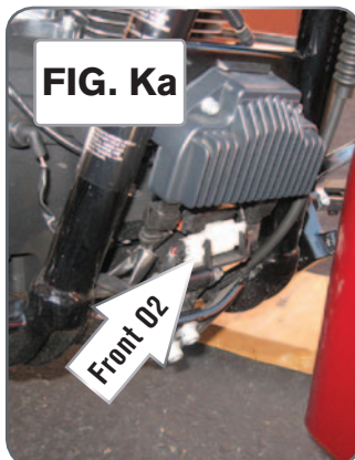
On 2006-2015 Dyna models the stock O2 connectors for the front cylinder are found at the front of the engine near the voltage regulator (Fig. Ka), and the rear cylinder O2 sensor connectors are found under the seat (Fig Kb).
