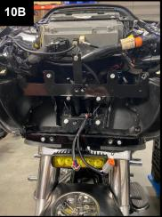
11. Connect the RG-HL-Y Wiring Adapter into the factory headlight connector (11A). Route RG-HL-Y Wiring Adapter behind the Mounting Plate (11B). Note: The two pin connector is designed for the Auxiliary Handlebar Mounted On/Off Switch CD P/N: CD-AUX-UNV (Sold Separately) to control the left side separately. It is recommended to have the Selective Yellow LED Fog Lamp controlled by the On/Off switch.
