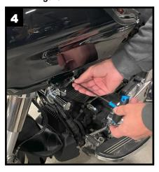
Remove both left and right lower T-25 Torx bolts from the bottom of each fairing chin spoiler.
